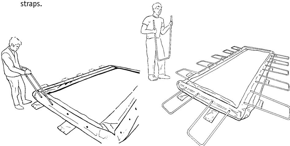
6. Starting from the four corners, thread steel pins **F** through foot straps and through stainless steel rings **G** of each "V" **D** pole (it is easier to do this operation if one person is inside the pool lifting a corner from a "V" pole **D** while another thread the steel pin **F** through foot strap).
