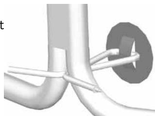
12. Turn around the white poles thus bringing near the two ends and insert the junction in the other end of the little transparent PVC pipe.
