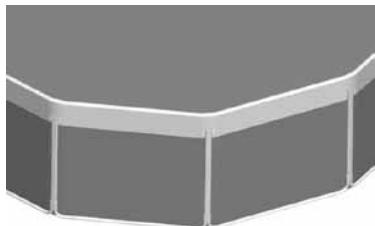
8. The curved ends of the upper pole **A** have to be inserted in the upper holes of the oval poles **B** on the structure previously assembled
