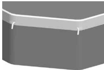
7. Insert the upper zinc-plated poles **A** in the upper pocket of the white top through the special opening leaving the two curved ends of the pole out.
