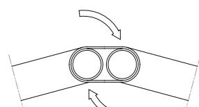
5. Complete the lower structure assembly joining all the pieces thus forming a closed circle.
