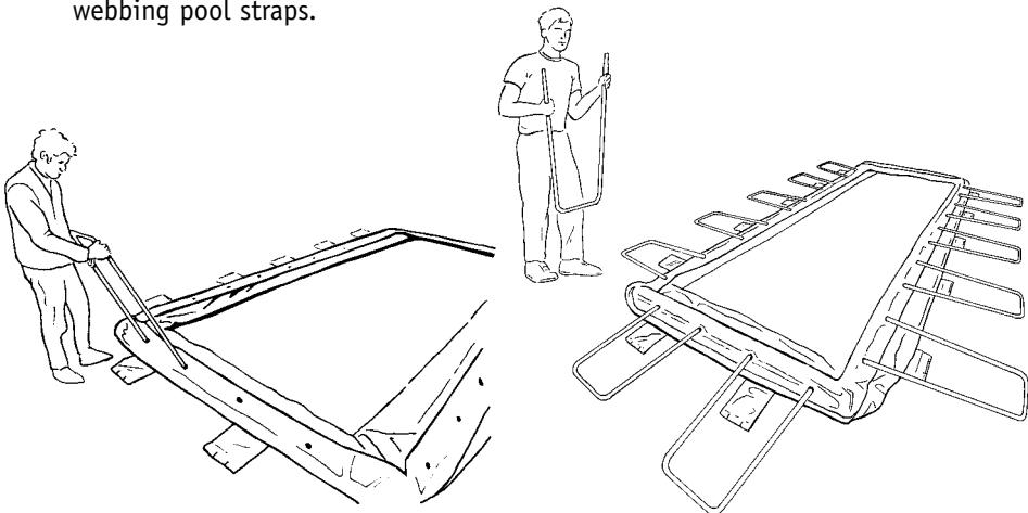
6. Starting from the four corners, thread steel pins F through foot straps and through inox rings G of each "V" D pole (it is easier to do this operation if one person is inside the pool lifting a corner from a "V" pole D while another thread the steel pin F through foot strap).
