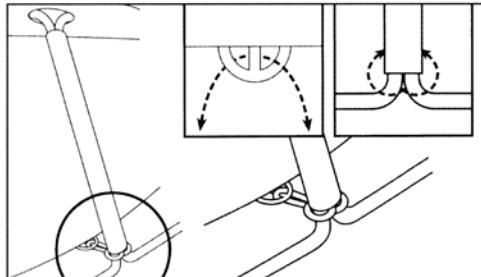
13. Once assembled the pool, pull each oval vertical white pole **B** and stretch the bottom of the pool in order to remove all the fold. The pool should have a regular polygonal shape.
