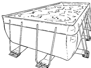
**WARNING:** When the pool is full it is not possible to pull the webbing straps of the supports to remove any creases in the bottom or move the legs if they are in the wrong position; the strain would damage the straps (remember always the huge weight of the water). In this case you must always empty out the pool first to make any adjustments.
