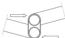
9. After inserting all the upper poles **A** turn each oval vertical pole once again as shown in the picture.
