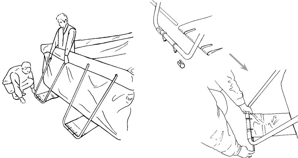
7. When all the steel pins are placed, while still inside of the pool, attach the Skimmer for the filtration system (*see filtration instructions*).
