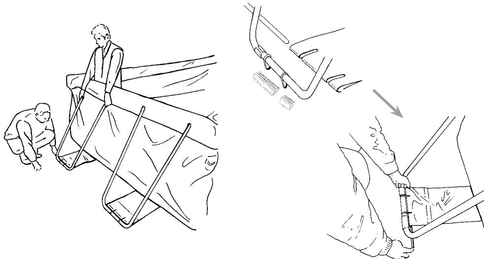
7. When all the steel pins **F** are placed, while still inside of the pool, attach the Skimmer for the filtration system (*see filtration instructions*).
